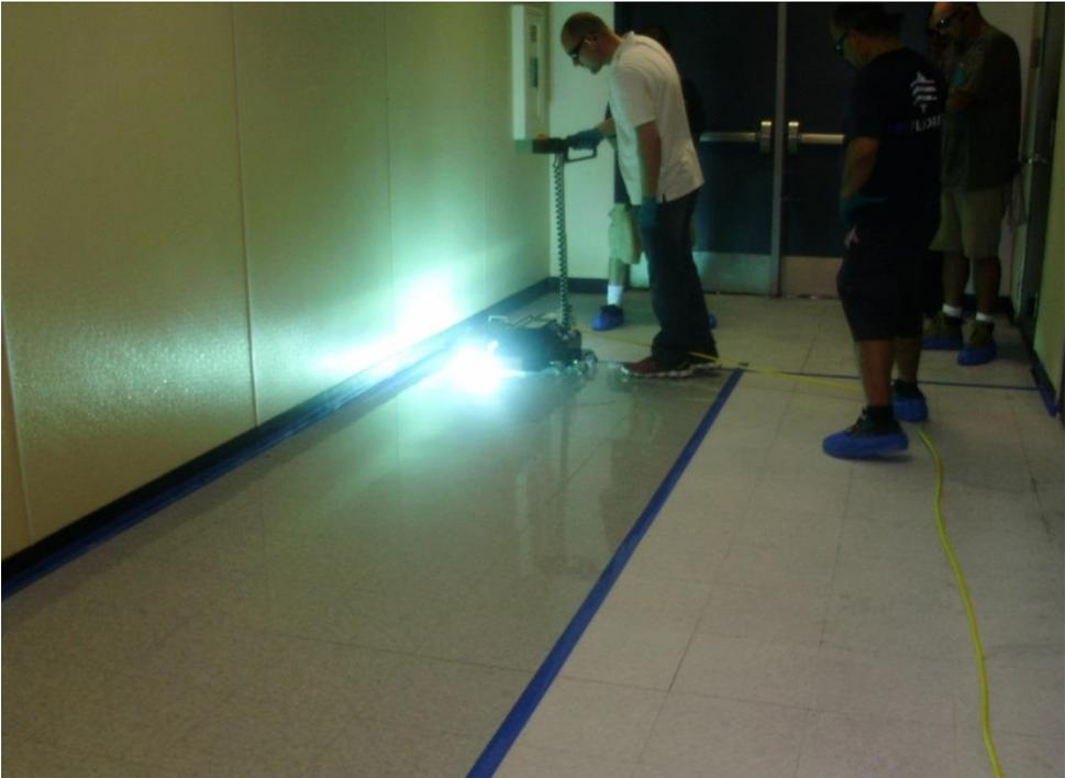
Figure 3-9. Floor Machine with UV Lights
