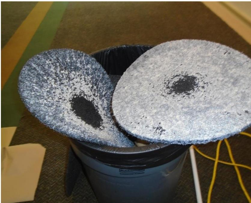
Figure 2-19. Picture of Hi-Pro and Regular Pad after Stripping at Irvine USD
