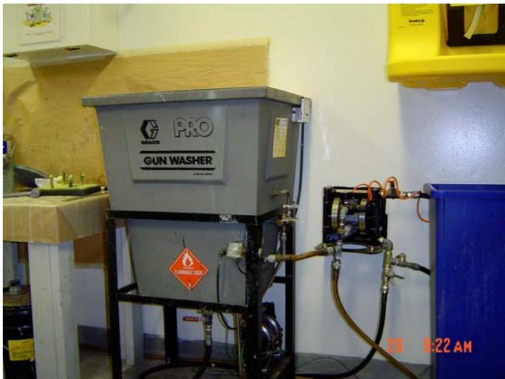
Figure 3-9. Typical Spray Gun Cleaning System
