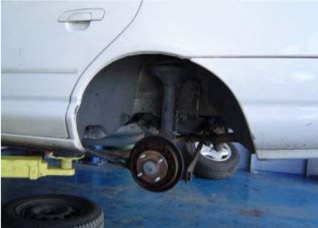
Figure 3-14. Vehicle with Drum Brakes.
