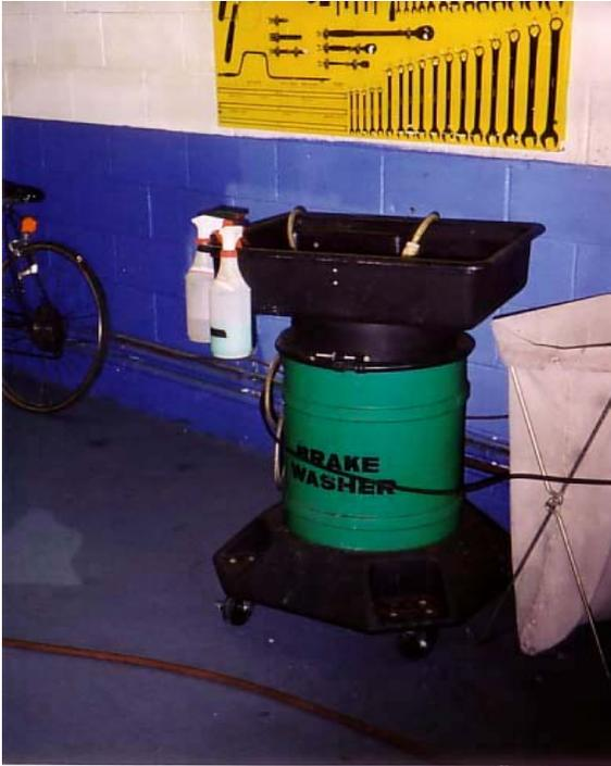
Figure 3-16. Brake Cleaning System
