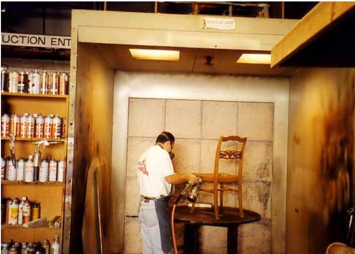
Figure 3-6. Typical Spray Booth at Wood Coating Operation
