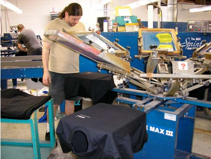
Figure 3-19. Automated Press for Textile Printing
