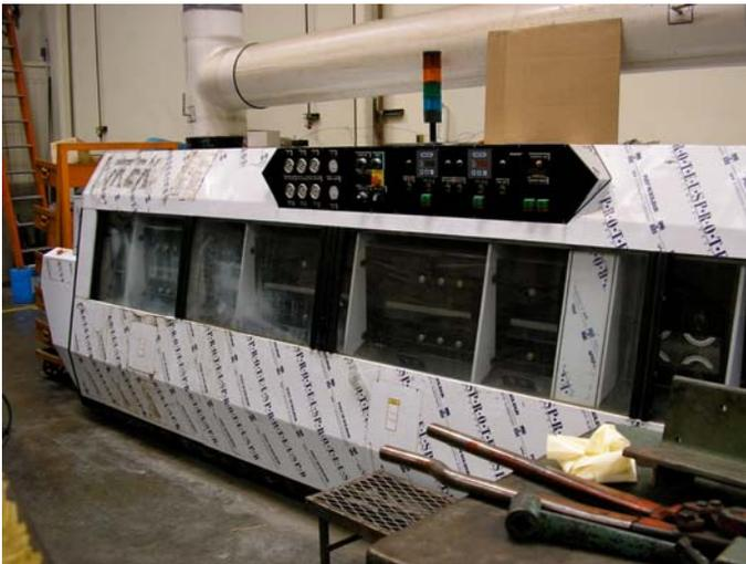
Figure 3-4. Conveyorized Water Board Cleaning System
