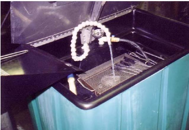
Figure 2-3. Immersion Parts Cleaner
