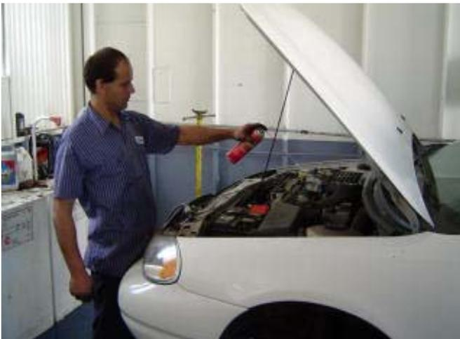
Figure 3-15. Technician Performing General Purpose Degreasing.
