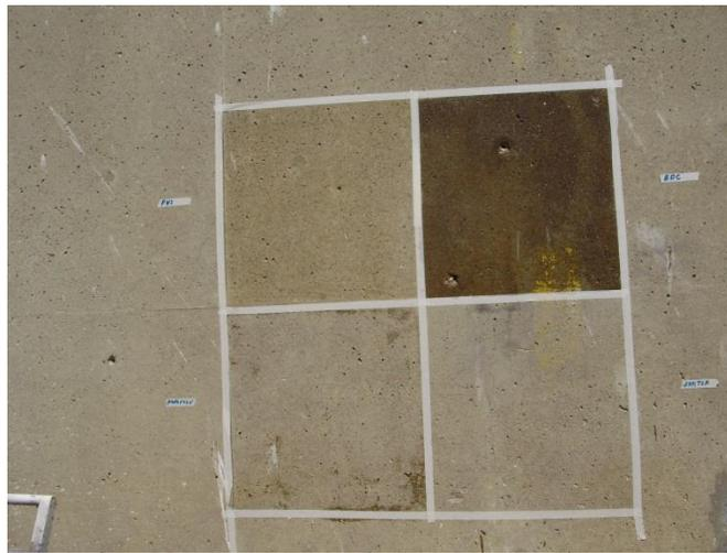
Figure 5-4. Graffiti resistant coatings on concrete wall
