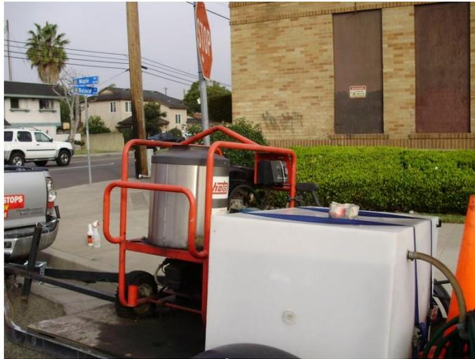
Figure 2-5. Soda blasting system
