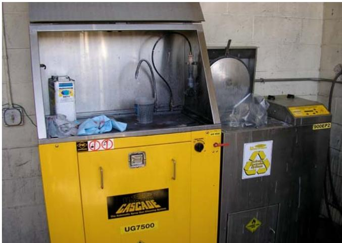
Figure 3-4. Typical Spray Gun Cleaning System
