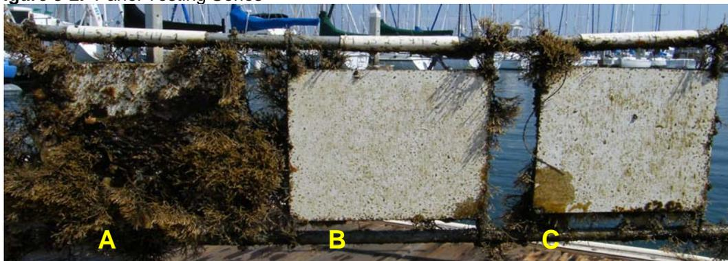
\* A = No Clean Panel; B = Standard Cleaning Panel; C = Manufacturer's Recommended Cleaning Panel
