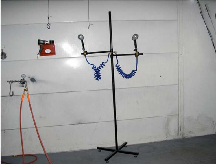
Figure 3-1. Typical Portable Hand-Held Dryer
