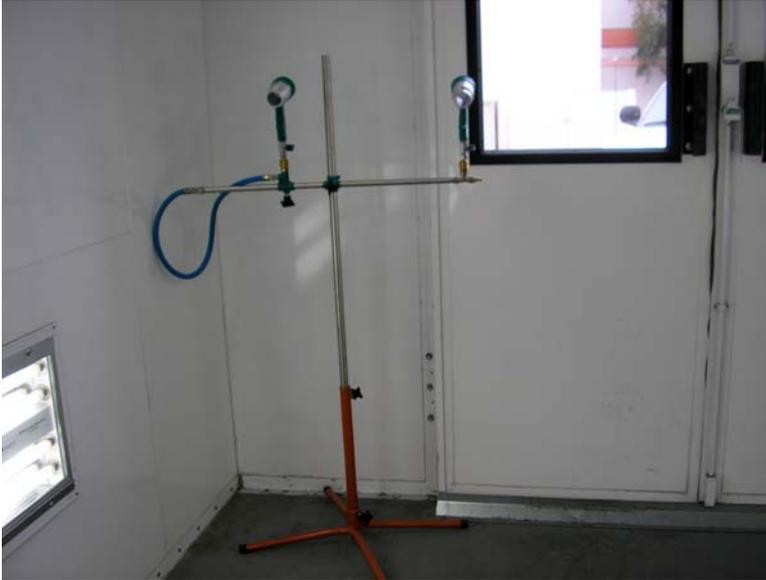
Figure 3-9. Portable Dryer at Autobody Shop #6
