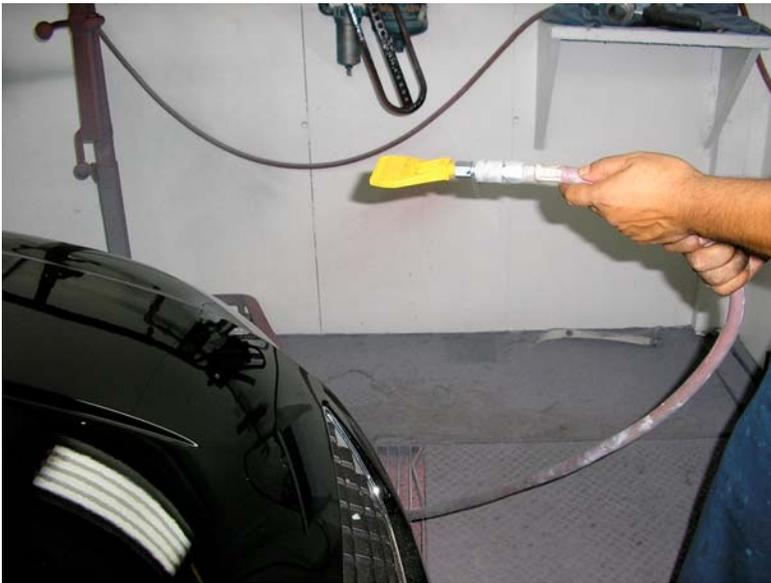
Figure 3-17. Painter Using Drying Tool
