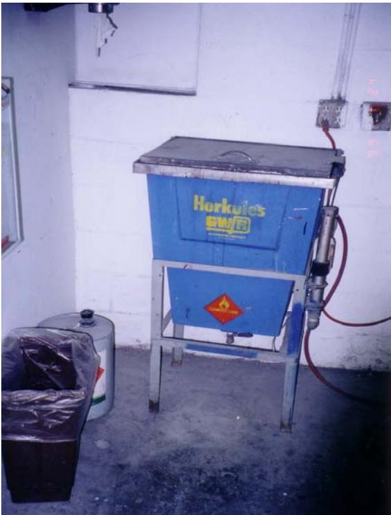
Figure 2-2. Spray Gun Cleaning Unit at Autobody Shop #2
