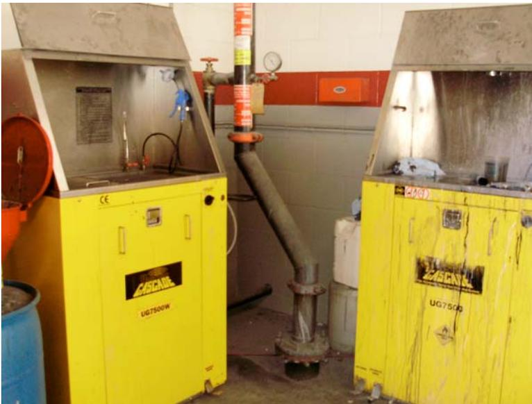
Figure 2-10. Solvent and Water Cleaning Systems at Autobody Shop #4
