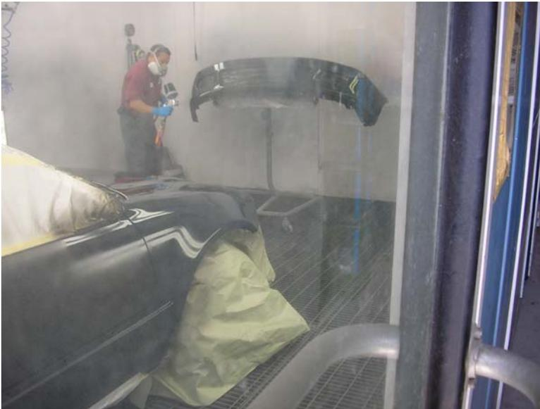
Figure 3-7. Painting Bumper with Waterborne Base Coat at Autobody Shop #4
