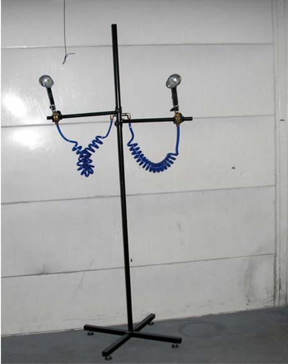
Figure 3-6. Portable Drying System at Autobody Shop#4
