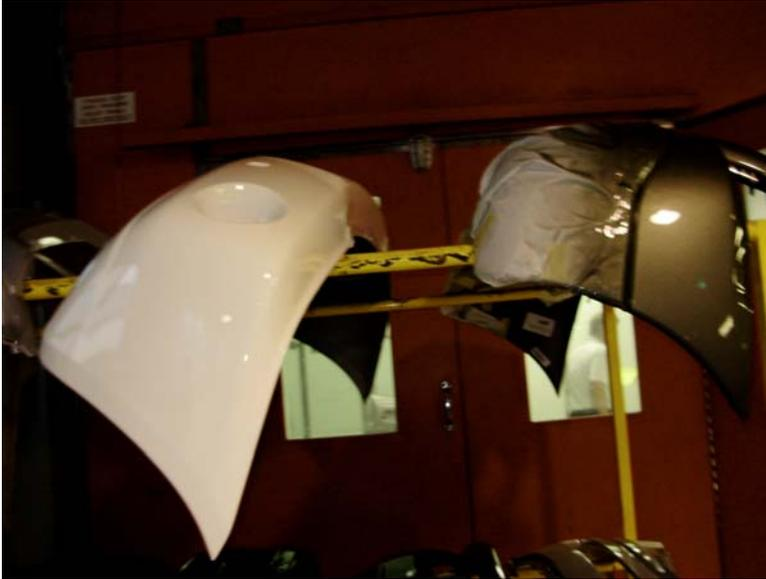
Figure 3-13. Parts Painted With Waterborne Base Coat at Autobody Shop #6
