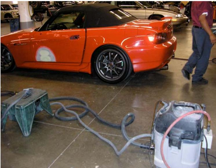
Figure 4-3. Typical Vacuum System Used with Mirka Sanding Discs
