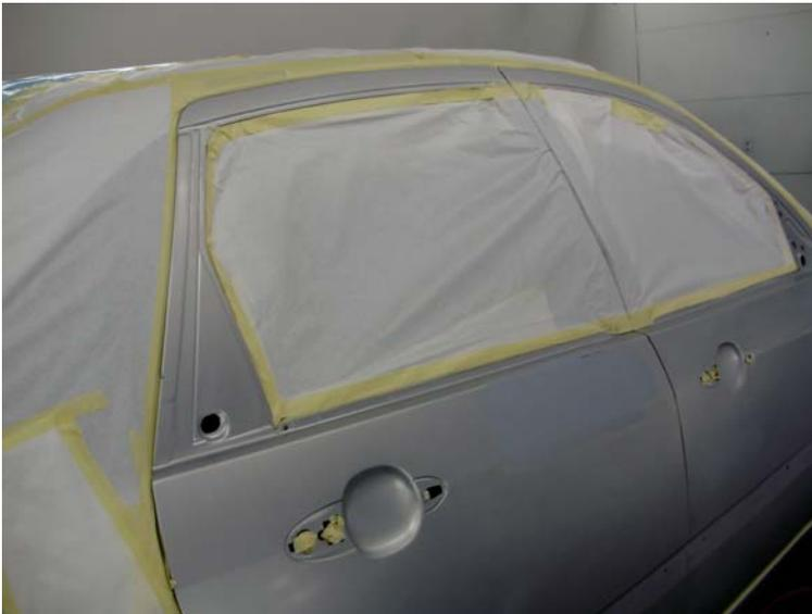
Figure 3-5. Car Prepped For Application of Waterborne Base Coat at Autobody Shop #4
