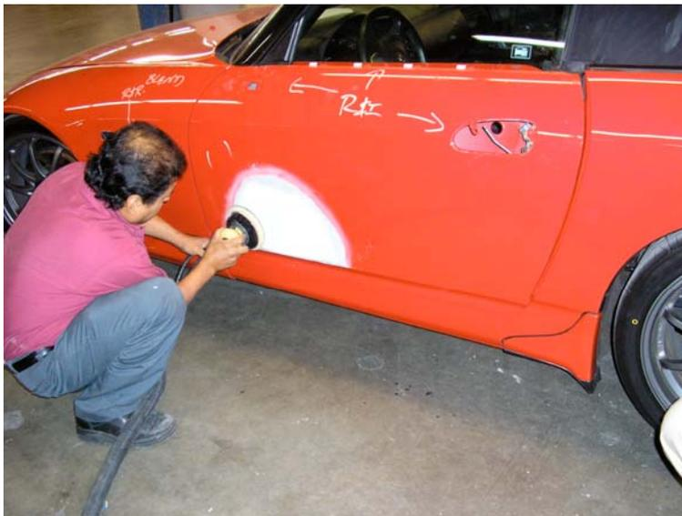
Figure 4-2. Sanding with Mirka Sanding Disc
