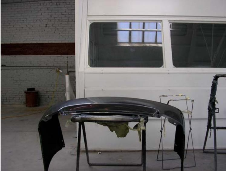
Figure 3-4. Car Bumper Painted with Waterborne Base Coat at Autobody Shop #4
