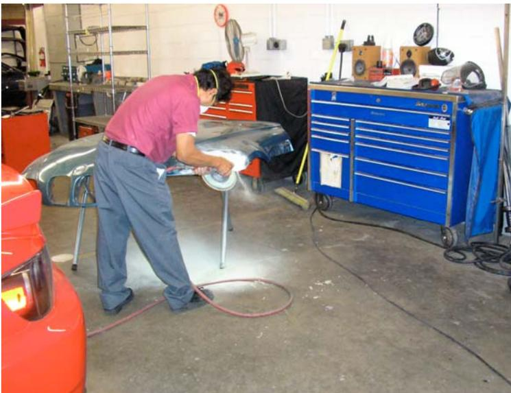
Figure 4-1. Sanding with Six Hole Sanding Disc
