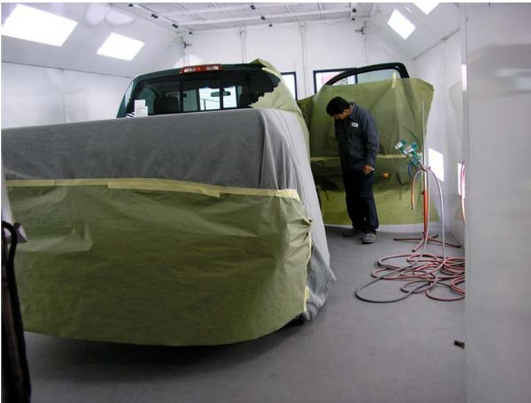
Figure 3-10. Painter Inspecting Truck Painted with Waterborne Base Coat at Autobody Shop #6
