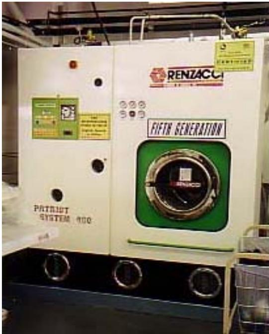
Figure 2-1. Typical PERC Machine
