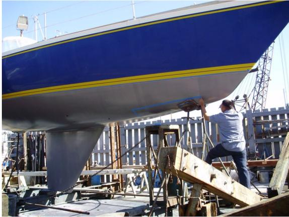
Diego to test biocide and nonbiocide alternatives to copper antifouling paints. One of the best performing nonbiocide paints in that project was a paint called Intersleek 900. The boat that was painted in December was painted with Intersleek 900. A sealer developed by International Paint was applied over the old copper paint and Intersleek 900 was applied over the sealer. The boat was painted at South Cost Shipyard in Newport Beach.
