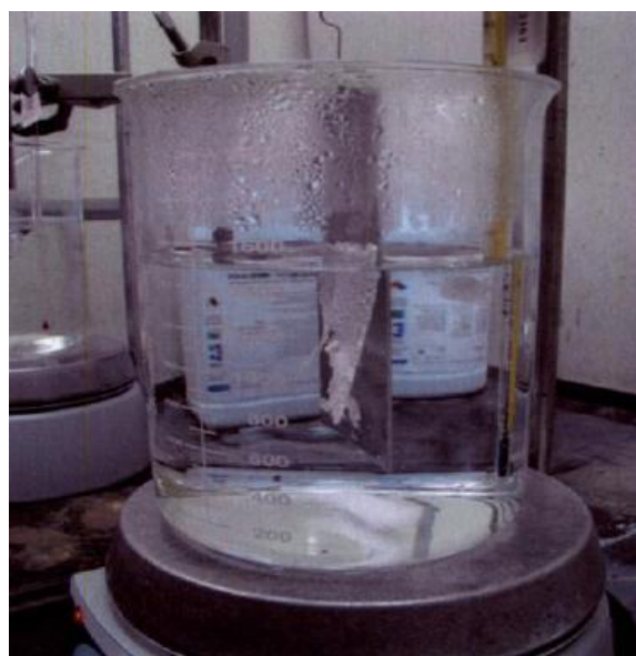
Figure 2-3. Soil Delaminating From Coupon
