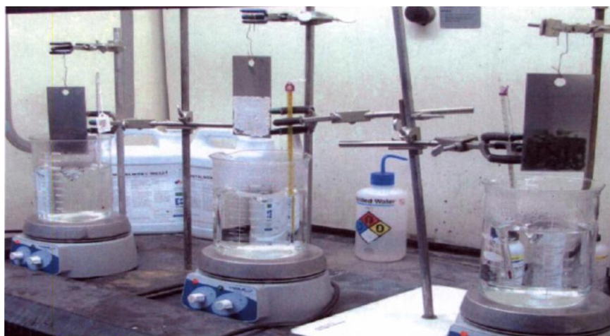
Figure 2-2. Beaker Setup For Coupon Tests
