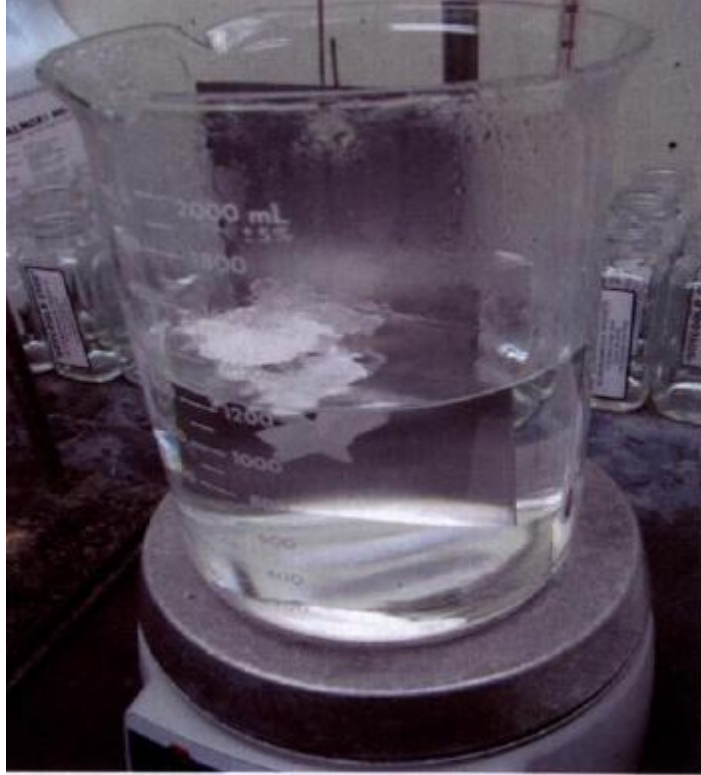
Figure 2-4. Soil Floating To Top Of Beaker
