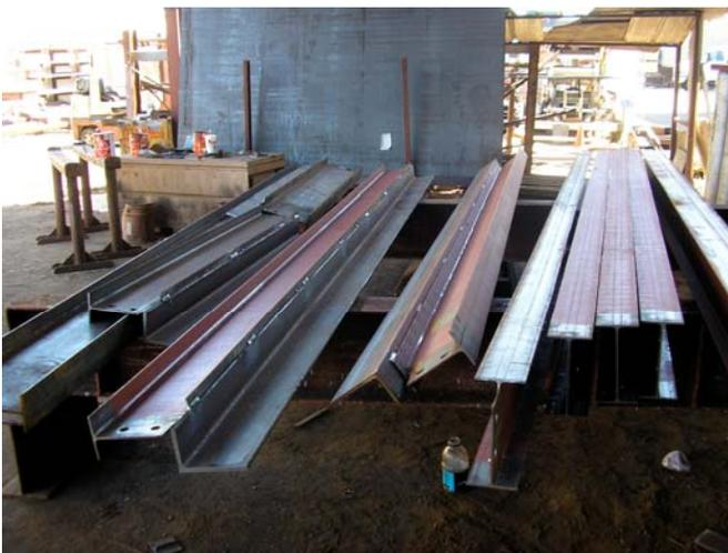
Figure 3-7. Steel Beams Coated by Contractor #2
