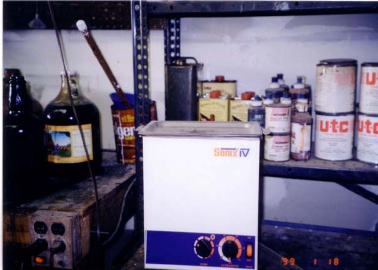
Figure 3-3. Ultrasonic Spray Gun Cleaning System
