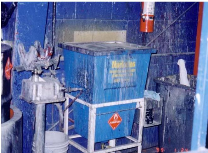
Figure 3-13. Spray Gun Cleaning System at Autobody Shop #3
