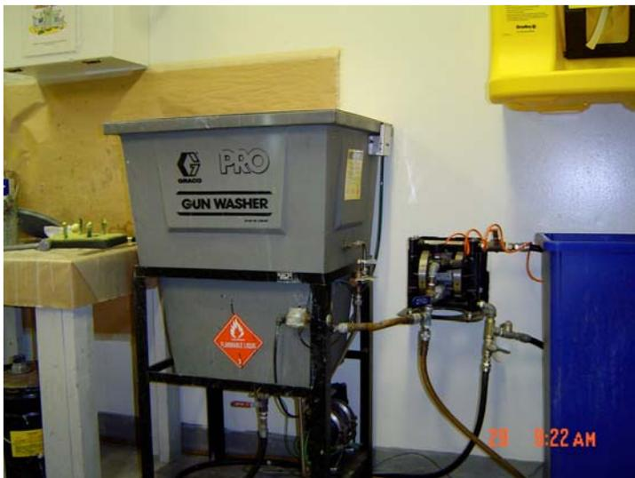
Figure 2-5. Typical Spray Gun Cleaning System
