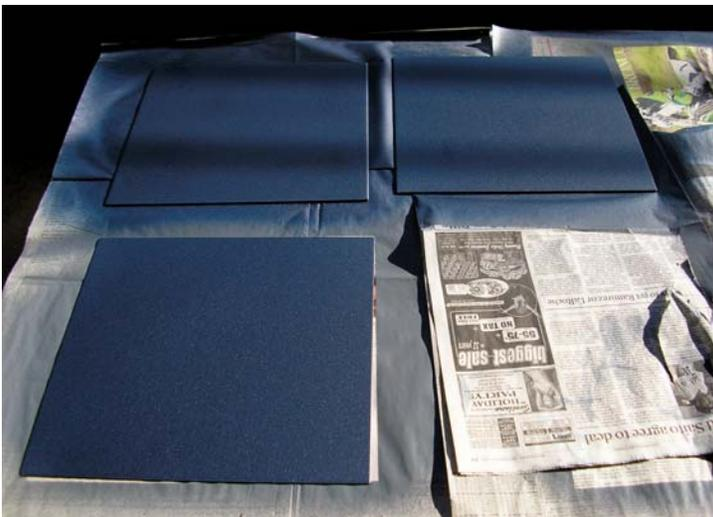
Figure 3-16. Panels After Base Coat Was Applied
