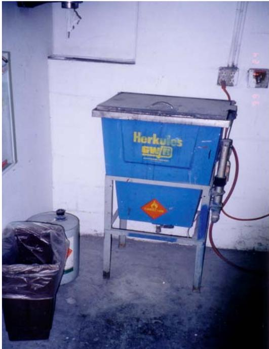
Figure 3-14. Spray Gun Cleaning System at Autobody Shop #4
